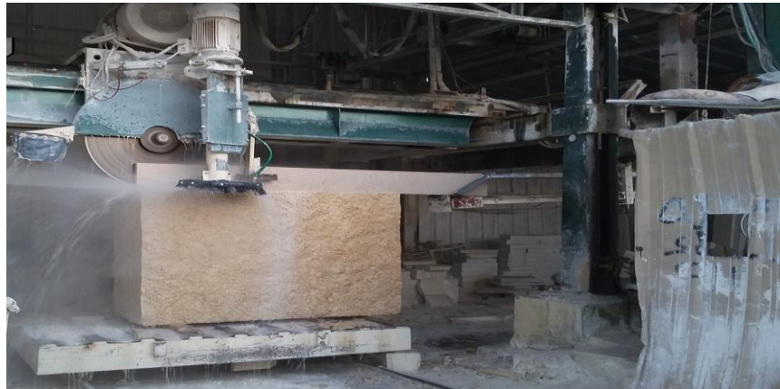
Figure (2) The use of water as a lubricator in the stone cutting process
