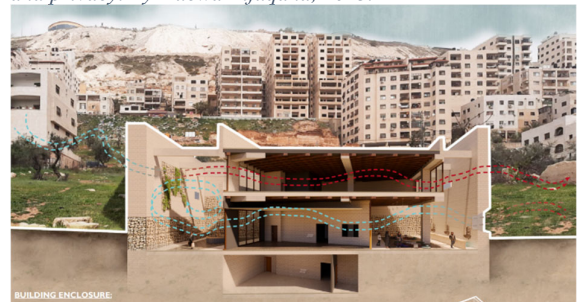
Figure 5. Demonstrating natural cooling using heat sinks and ventilated enclosures. By Julien Yray, 2023.
