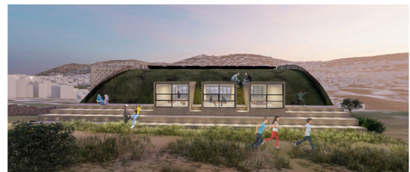
Figure 4. Earth-sheltered structure to provide natural cooling and privacy. By Duewa Alfuqaha, 2023.
