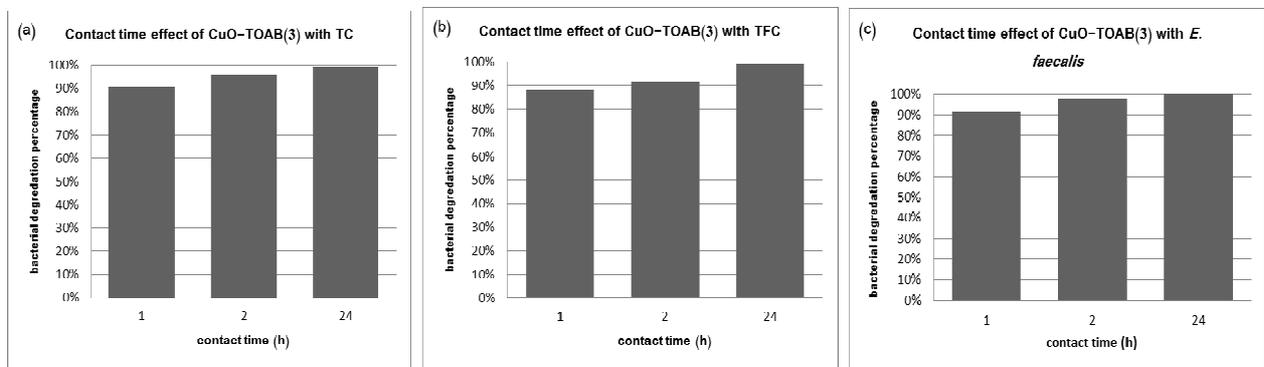
Fig.14: Contact time of 1, 2 and 24 h effect for CuO-TOAB(3) with a) TC b) FC c) *E. faecalis*
