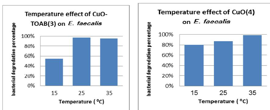
**Fig.17:** The effect of wastewater temperature (15, 25 and 35 °C) on degradation percentage of *E. faecalis* using a) CuO-TOAB(3) and b) CuO(4).
