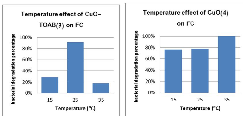
**Fig.16:** The effect of wastewater temperature (15, 25 and 35 °C) on degradation percentage of FC using a) CuO-TOAB(3) and b) CuO(4).
