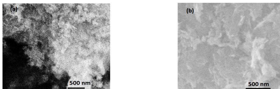
**Fig. 5:** SEM images of CuO nanoparticles prepared at 75 °C a) with TOAB surfactant b) without TOAB surfactant.
