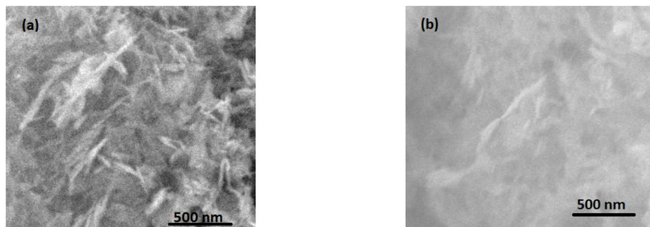
**Fig. 4:** SEM images of CuO nanoparticles prepared at 65 °C a) with TOAB surfactant b) without TOAB surfactant
