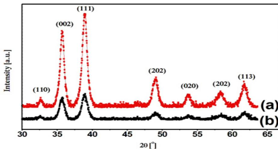
Fig. 3: XRD pattern of CuO nanoparticles prepared at 85 °C a) without TOAB surfactant b) with TOAB surfactant.
