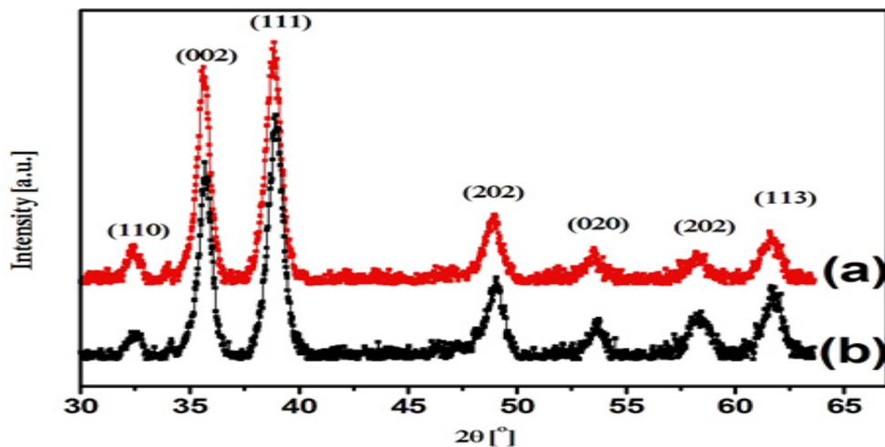
Fig. 1: XRD pattern of CuO nanoparticles prepared at 65 °C a) without TOAB surfactant b) with TOAB surfactant.
