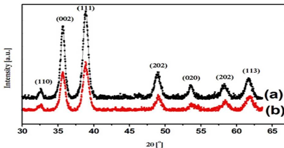
Fig. 2: XRD pattern of CuO nanoparticles prepared at 75 °C a) without TOAB surfactant b) with TOAB surfactant.
