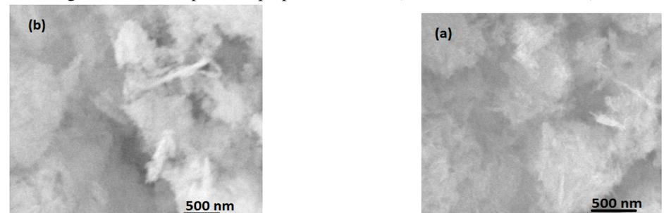
**Fig. 6:** SEM images of CuO nanoparticles prepared at 85 °C a) with TOAB surfactant b) without TOAB surfactant.
