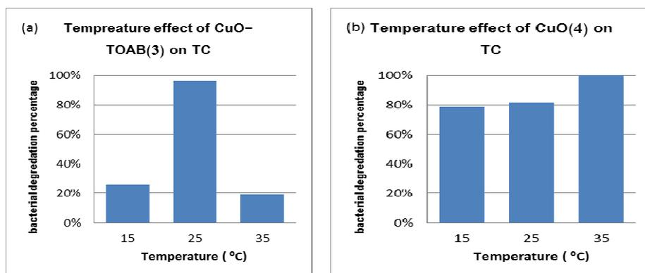
Fig.15: The effect of wastewater temperature (15, 25 and 35 °C) on degradation percentage of TC using a) CuO-TOAB(3) and b) CuO(4).
