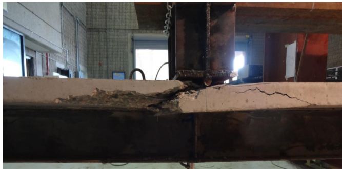
Fig. 23. Girder G1 shear compression failure
