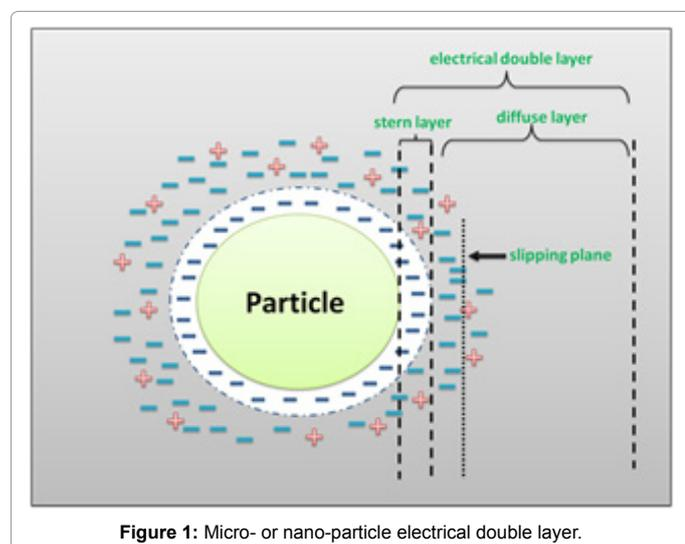
Figure 1: Micro- or nano-particle electrical double layer.
