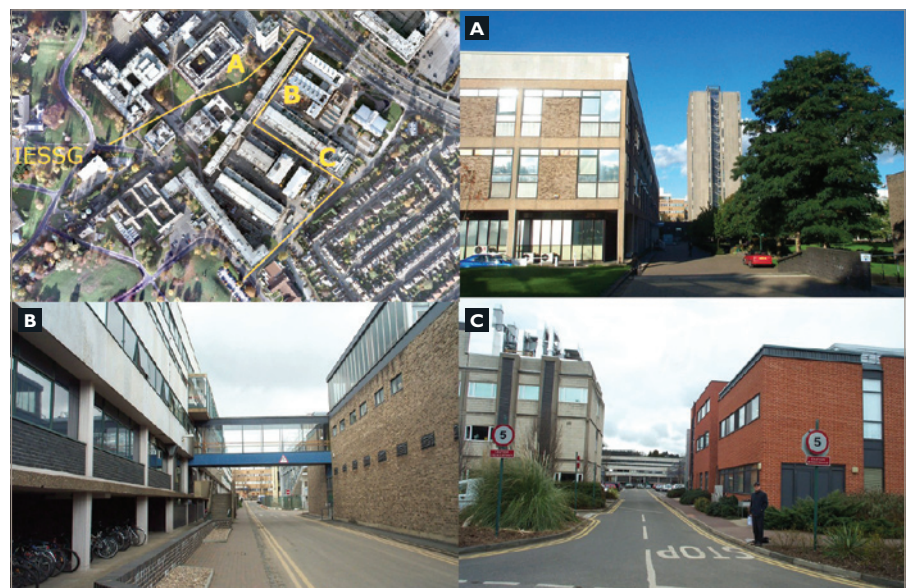
Figure 5. The GNSS test network at the University of Nottingham campus includes a variety of difficult 'urban' scenarios including tall buildings (A), urban canyons (B) and bridges (C)
