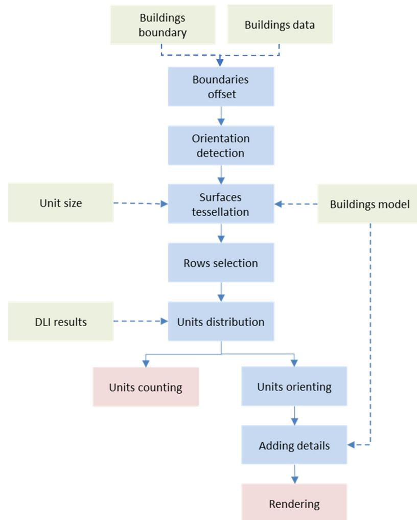
Figure 24. AGRI|gen\Design tool general algorithm (Diagram: Ghazal 2020).
