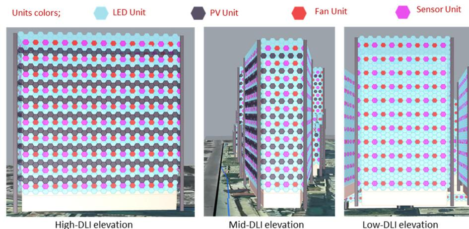
**Figure 36.** Different distribution patterns on facades with different DLI values (Diagram: Ghazal 2020).
