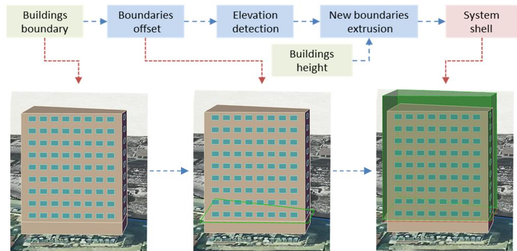
Figure 25. Shell modelling algorithm and results (Photos and Diagram: Ghazal 2020).
