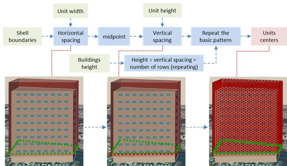
Figure 26. Facade tessellation Shell algorithm and results (Photos and Diagram: Ghazal 2020).
