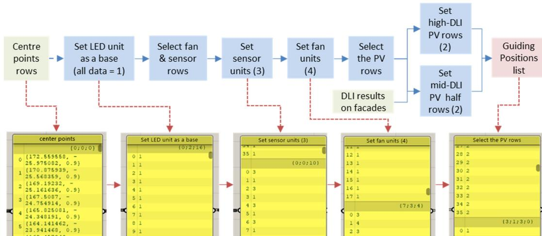
Figure 30. Implementing distribution rules algorithm (Photos and Diagram: Ghazal 2020).
