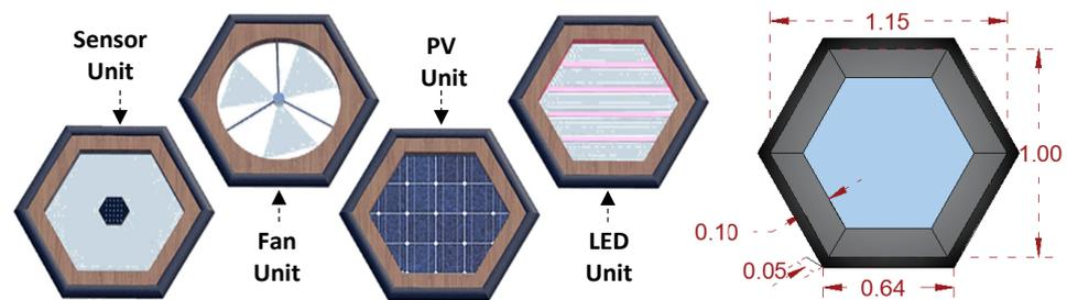
Figure 23. Unites types and dimensions (Diagram: Ghazal 2020).
