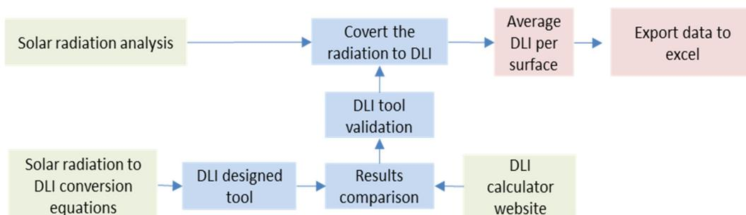
**Figure 16.** DLI calculation algorithm (Diagram: Ghazal 2020).
