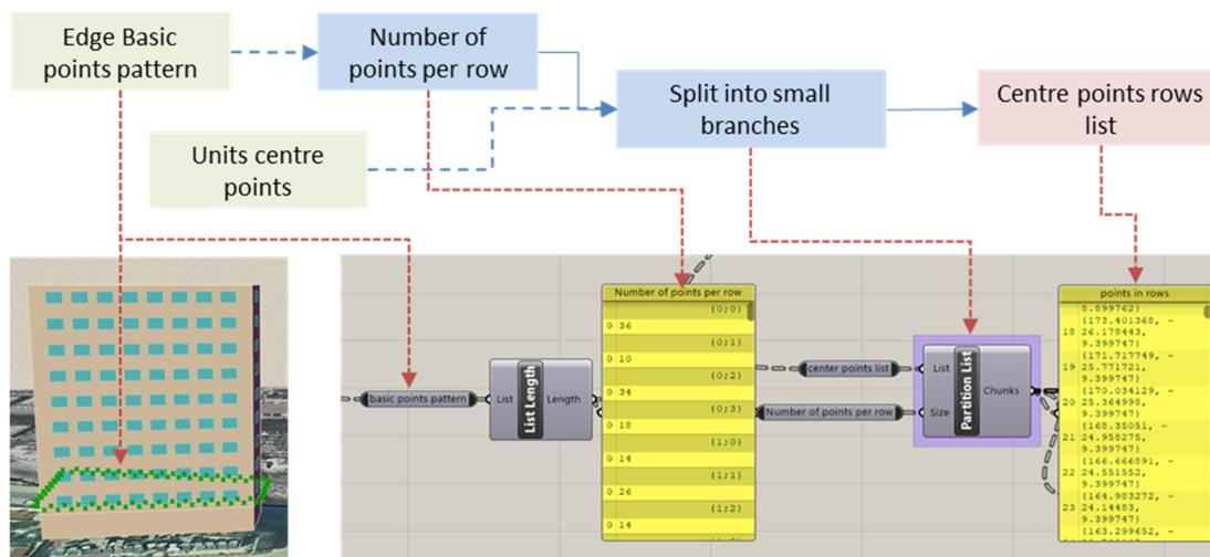
Figure 29. Rows selection algorithm (Photos and Diagram: Ghazal 2020).
