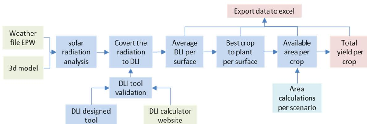
**Figure 14.** Neighbourhood Production analysis algorithm (Diagram: Ghazal 2020).
