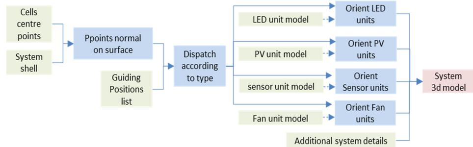
Figure 32. Units orientation algorithm (Photos and Diagrams: Ghazal 2020).
