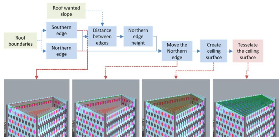
Figure 34. Roof Design algorithm and results (Photos and Diagram: Ghazal 2020).
