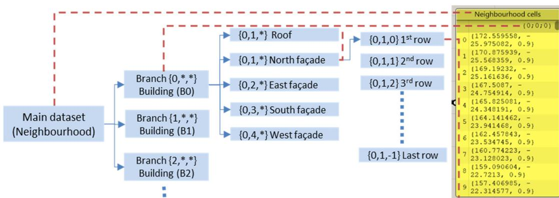
Figure 31. The used data tree structure to deliver different information across the Grasshopper workflow (Diagram: Ghazal 2020).
