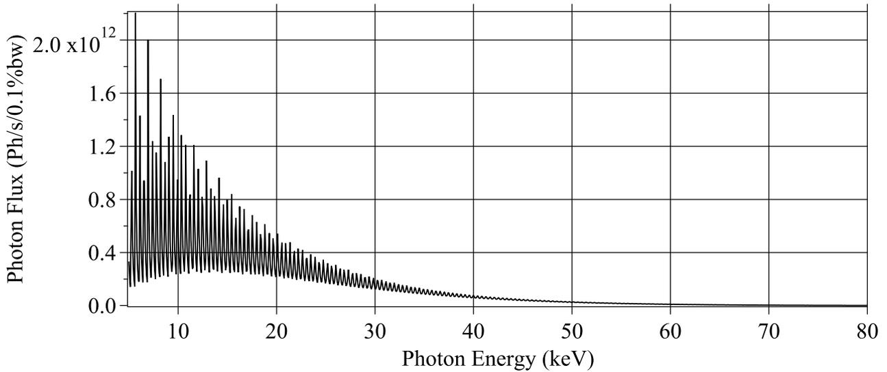
FIG. 7: Photon flux of the first proposed wiggler ( $\lambda_0 = 98$  mm) in the wiggler regime calculated by SRW at 10 m from the source through an aperture of  $0.1 \times 0.1$  mm<sup>2</sup>. The wiggler is set at gap 14.7 mm. The magnetic field  $B=1.78$  T. The electron beam parameters are:  $E = 2.739$  GeV,  $I = 500$  mA,  $\beta_x = 4.6$  m,  $\beta_z = 2.2$  m,  $\epsilon_x = 3.9$  nm.rad,  $\epsilon_z = 39$  pm.rad,  $\sigma_e = 0.1\%$ .
