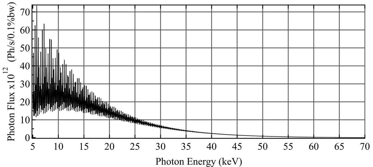
FIG. 5: Photon flux of the first proposed wiggler ( $\lambda_0 = 164$  mm) in the wiggler regime calculated by SRW at 10 m from the source through an aperture of  $0.1 \times 0.1$  mm<sup>2</sup>. The wiggler is set at gap 14.7 mm. The field B=1.65 T. The electron beam parameters are:  $E = 2.739$  GeV,  $I = 500$  mA,  $\beta_x = 4.6$  m,  $\beta_z = 2.2$  m,  $\epsilon_x = 3.9$  nm.rad,  $\epsilon_z = 39$  pm.rad,  $\sigma_e = 0.1\%$ .
