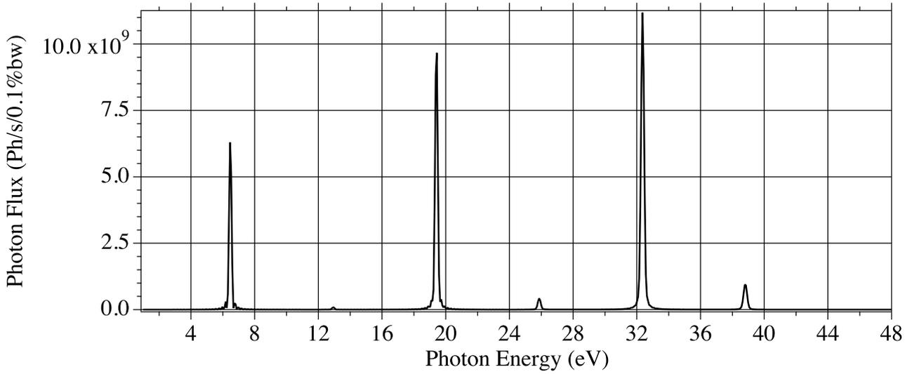
FIG. 6: Photon flux of the first proposed wiggler ( $\lambda_0 = 98$  mm) in the undulator regime calculated by SRW at 10 m from the source through an aperture of  $0.1 \times 0.1$  mm<sup>2</sup>. The wiggler is set at gap 16.7 mm. The magnetic field  $B=1.63$  T. The electron beam parameters are:  $E = 2.739$  GeV,  $I = 500$  mA,  $\beta_x = 4.6$  m,  $\beta_z = 2.2$  m,  $\epsilon_x = 3.9$  nm.rad,  $\epsilon_z = 39$  pm.rad,  $\sigma_e = 0.1\%$ .
