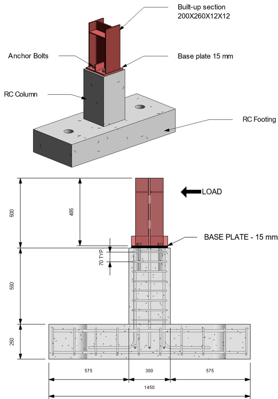
**Figure 2.** Details of geometry and anchorage of constructed specimens.
