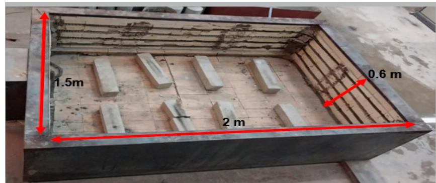
**Figure 5.** The oven used to apply high temperature.
