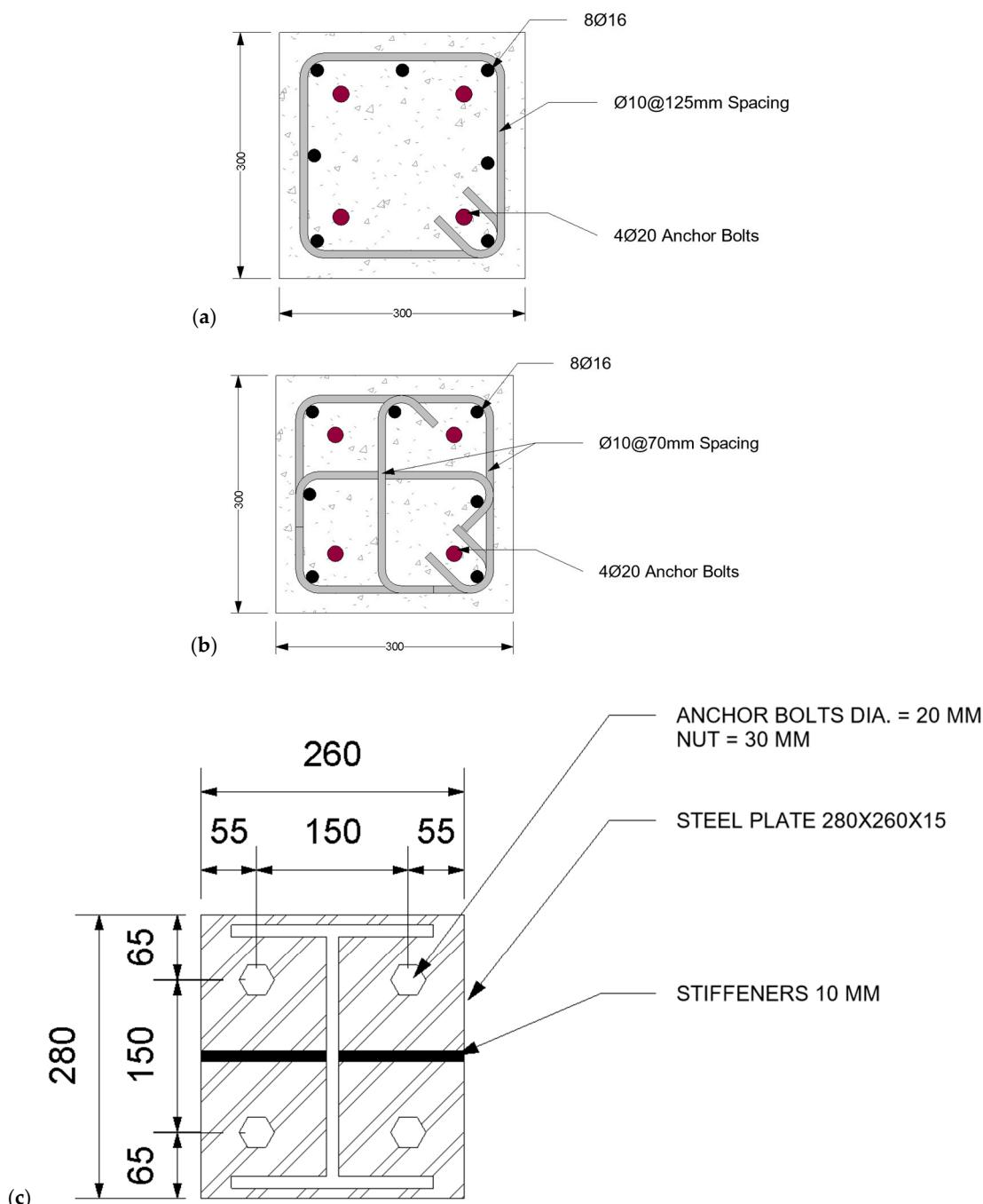
**Figure 3.** Details of (a) reinforcement based on IMF specifications, (b) reinforcement based on SMF specifications, and (c) anchorage of all specimens.
