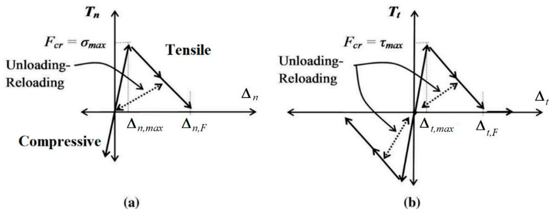
**Figure 12.** Material laws for cohesive zone material model under (a) pure normal and (b) pure shear stresses.
