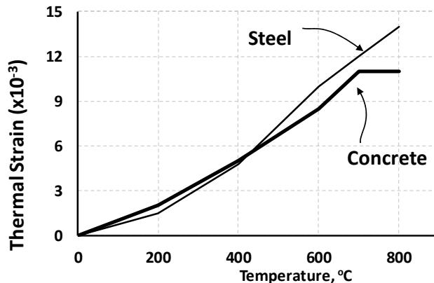
**Figure 11.** Thermal strain for all types of steel and for concrete.
