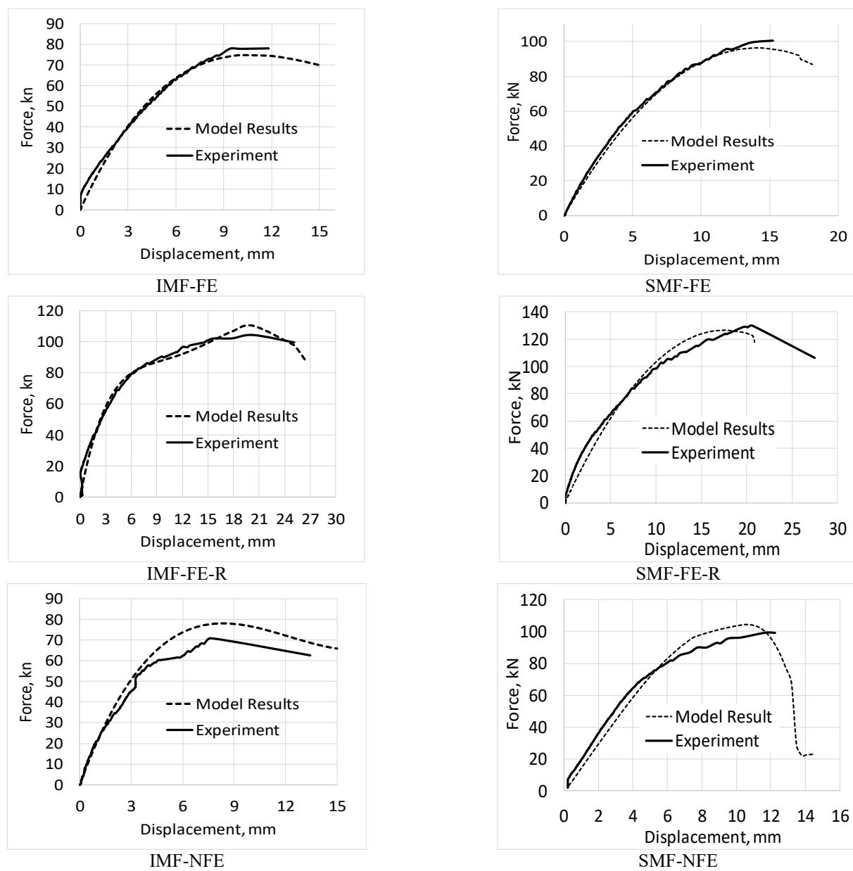
**Figure 8.** Comparing predictions from the FE model against the experimental results.
