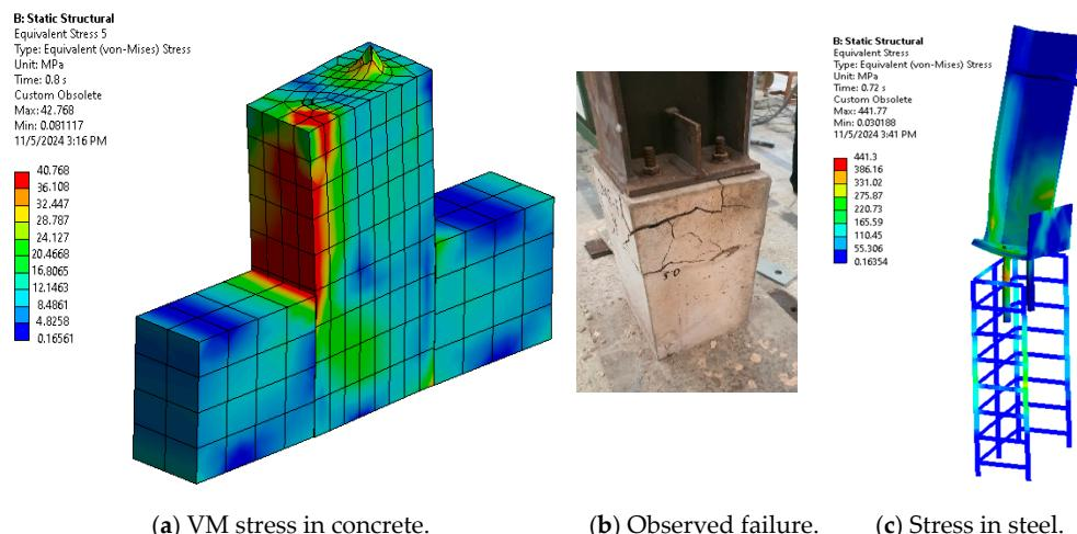
**Figure 14.** Comparing results for the specimen IMF-FE and (a) von-Mises equivalent stresses at time of failure, where the crushing is shown to happen near the compressed region; (b) the observed failure pattern; and (c) stresses in the steel, anchor bolts, and reinforcement. While the anchor rods and structural steel reached the yielding point, the reinforcement remained elastic.
