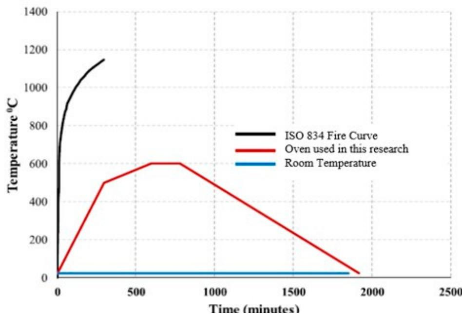
**Figure 6.** Time–temperature curves of heat-exposed specimens.
