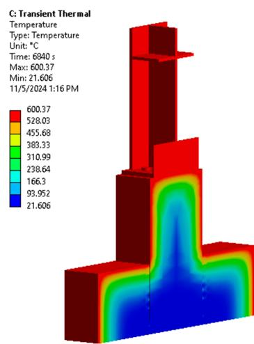
**Figure 13.** Cross-sectional temperature distribution (°C) from the thermal analysis after 3 h in the furnace.
