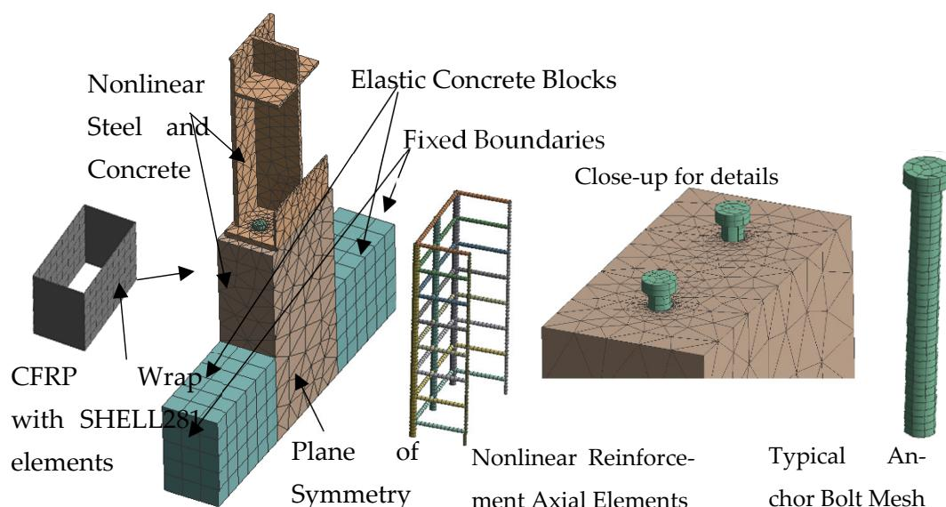
**Figure 9.** Mesh details for the finite-element half-model.
