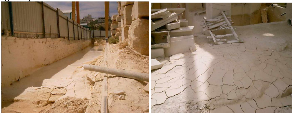
Figure 1: photographs of stone cutting waste sludge
